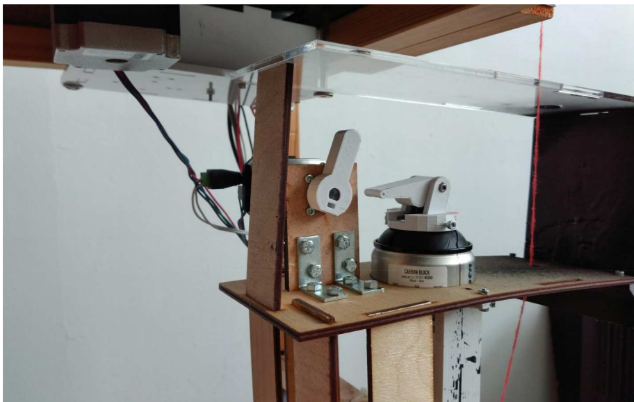
Figure 7. The custom-made yarn dyeing mechanism activated during peaks of attention.
